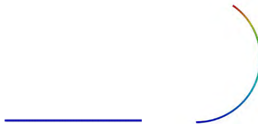
Figure 1. Undeformed and deformed configuration of a thin cantilever beam subject to pure bending
