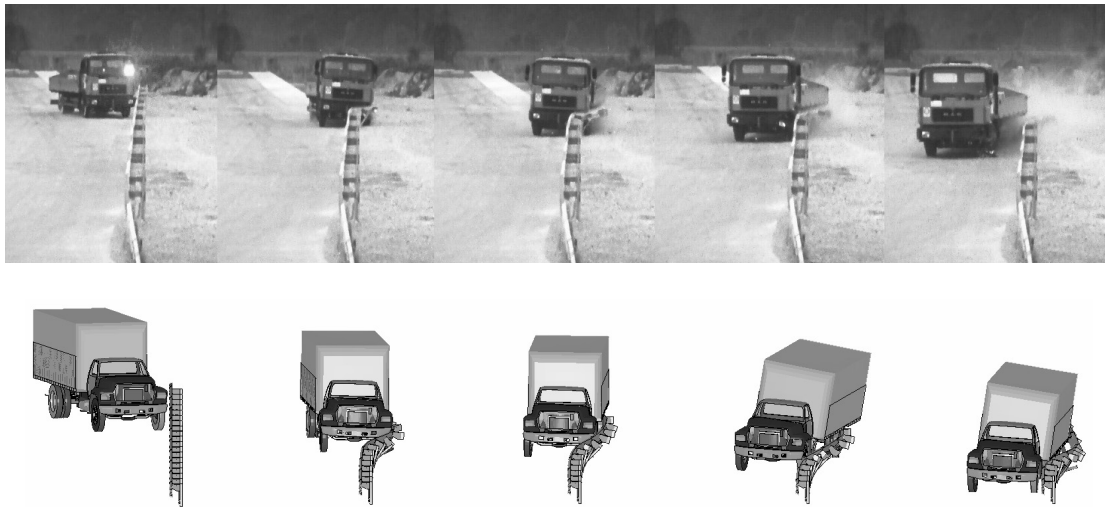
Figure 1. The barrier deformation during large scale test (top) and simulation (bottom)
