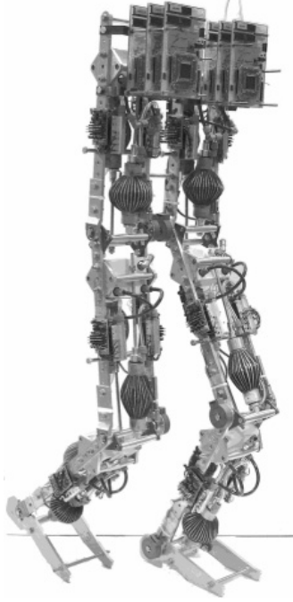
Fig. 11: Bipedal walking robot “Lucy” actuated by PPAM’s
