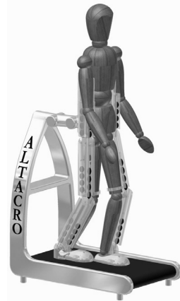
Fig. 17. Artistic view of the step rehabilitation robot actuated by PPAM’s
