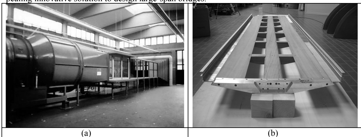
Figure 1. CRIACIV Boundary Layer Wind Tunnel, Italy (a); picture of one of the multiple-box girder deck section models tested in wind tunnel (b)
