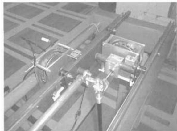
Figure 2: Experimental model setup with two damping units
