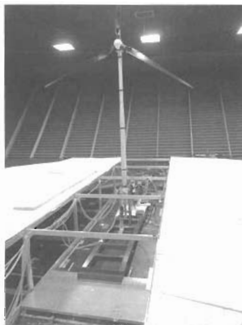
Figure 1. Experimental rig for testing offshore wind turbines within a wind tunnel facility
