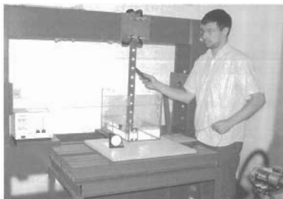
Figure 2. Impact test on the cantilever beam immersed in water and response is measured by laser vibrometer
