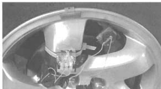
Figure 4. WTPMS device mounted on the car tire rim.
