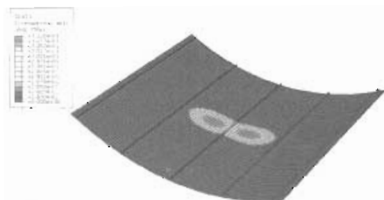
Figure 2. Micromechanics of Failure criterion for a static tensile load case.
