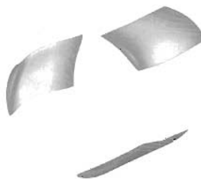
Figure 1. Post processed results of a simulation; the streamlines represent the stream velocity and blade deformations are 20× enlarged.
